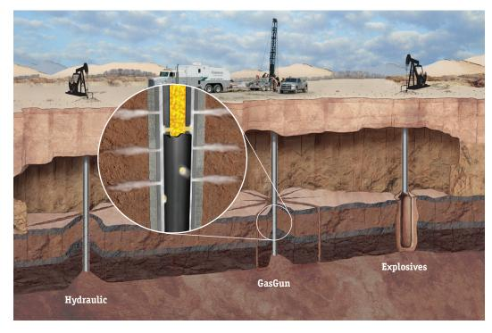
ing. Call it a low explosive. It generates high-pressure gas at a rapid rate that is tailored to the formation's characteristics. The rate is fast enough to create multiple fractures radiating 10 to 50 feet from the wellbore, but not so rapid as to pulverize and compact the rock — which is the danger of using classic high explosives such as nitroglycerine.
